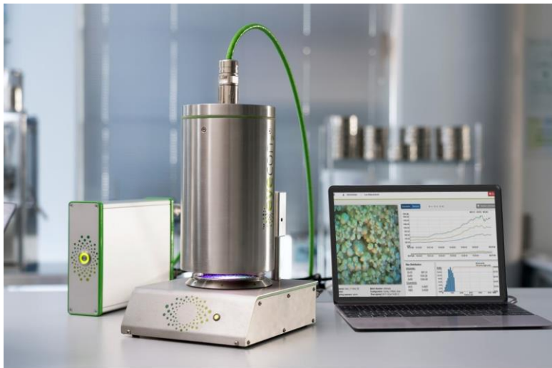
Figure 2: The Eyecon 2 particle characteriser setup at-line
