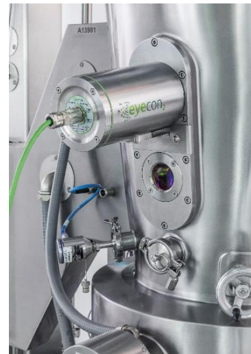
Figure 1: The Eyecon 2 particle characteriser setup In-line on a GPCG30 Fluid bed
